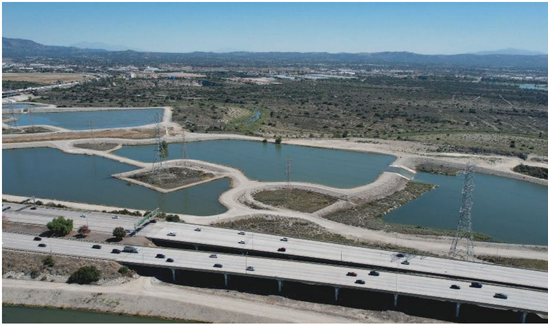
At far left and above is the Puente Valley Intermediate Zone Remedy Operating Unit, which is one of 32 active groundwater treatment facilities that are integral to the cleanup coordinated by the San Gabriel Basin Water Quality Authority. At left, the water percolates into the groundwater basin from the Santa Fe Spreading Grounds near the 210-605 freeway interchange.
