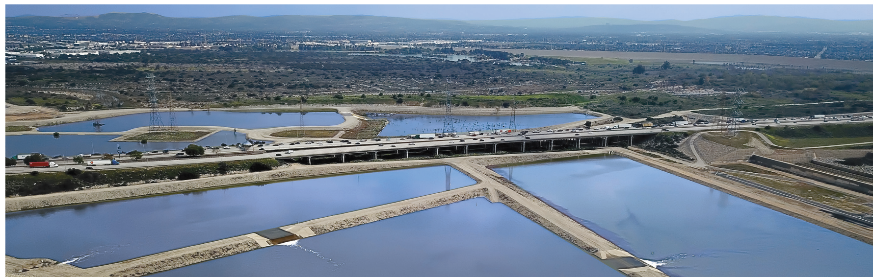
Above, water percolates into the Main San Gabriel Basin from the Santa Fe Spreading Grounds near the 210-605 freeway interchange. At right, the South Pasadena Wilson Treatment Facility is one of 32 active groundwater treatment plants that are integral to the cleanup coordinated by the San Gabriel Basin Water Quality Authority.
